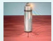
Fig 10 shows the deployment of tines into the myocardium during implant.
